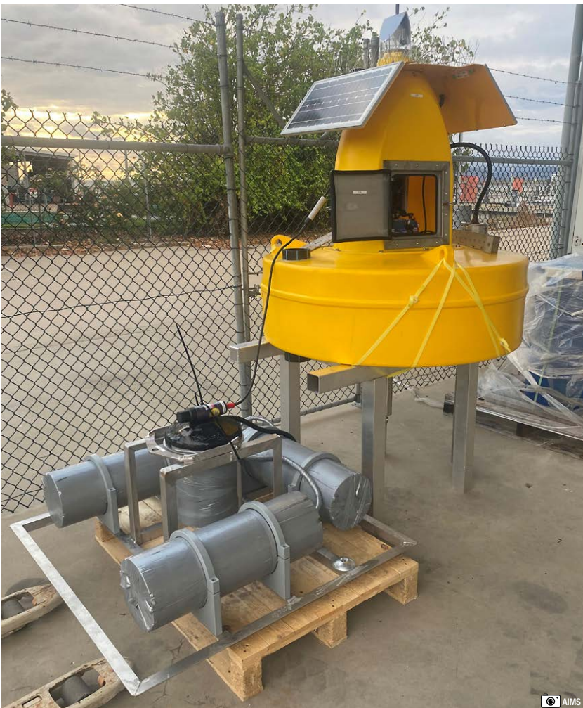
Figure 6: Subsea (Sonardyne Origin 600) and topside (Sonardyne "Nano" modem attached to YSI DB600 water quality Xylem buoy) instrumentation set-up for real-time reporting of oceanographic data on the ReefWorks range.
