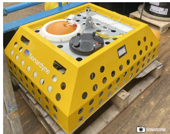
Figure 2: Integrated seabed sensor node housing the Origin 600 ADCP delivered by Sonardyne for SSCS.
