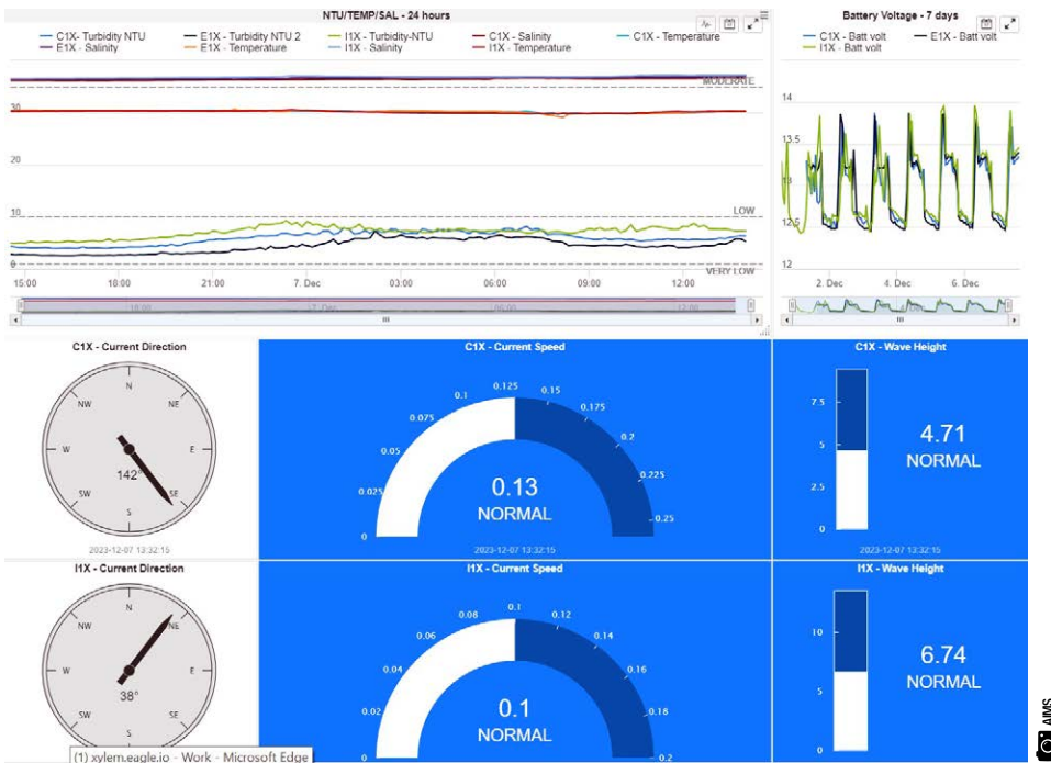
Figure 7: Example screenshot of the Eagle.io dashboard showing real-time data displayed for a range of oceanographic parameters, including currents, waves, turbidity, temperature, and salinity.
